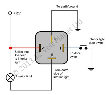
**Note:** The interior light earth connection is split and connected between terminals 3 & 5
